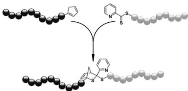
Scheme 12 General synthetic strategy for producing well-defined high M_n block copolymers via the RAFT–HDA click reaction (TFA, CHCl 3 , RT). 84
