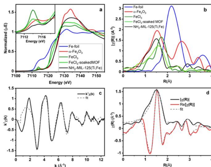
Figure 2. Fe K-edge a) XANES, b) EXAFS spectra and c) k-space and d) R-space  $\text{NH}_2\text{-MIL-125(Ti, Fe)}$  EXAFS spectrum and corresponding fit.
