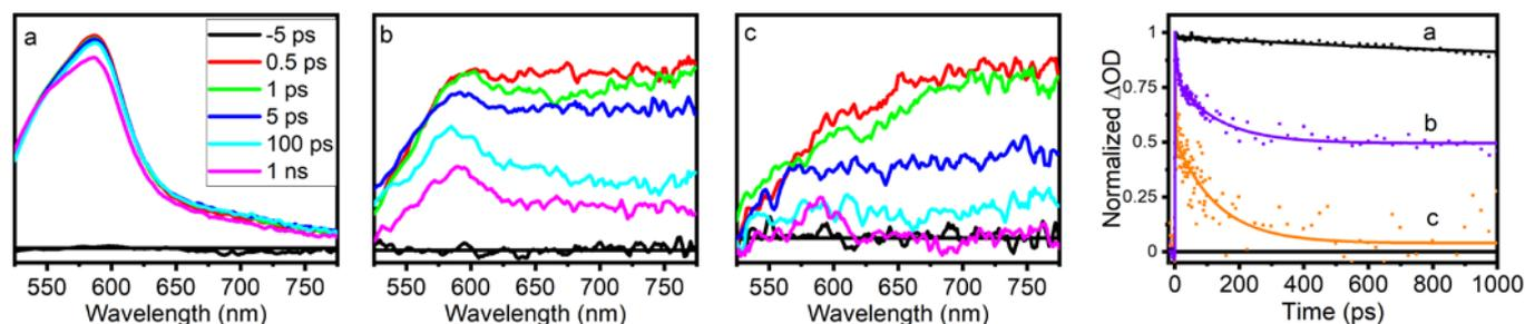
Figure 3. Optical transient absorption spectra and kinetics (collected at 585 nm) of a)  $\text{NH}_2\text{-BDC}$ , b)  $\text{NH}_2\text{-MIL-125(Ti,Fe)}$ , and c)  $\text{NH}_2\text{-MIL-125(Ti)}$ .
