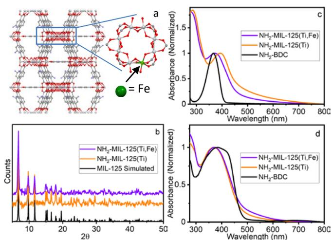
Figure 1. a) Proposed structure of  $\text{NH}_2\text{-MIL-125(Ti, Fe)}$ , b) PXRD, c) UV-vis absorption and d) DR spectra of  $\text{NH}_2\text{-BDC}$ ,  $\text{NH}_2\text{-MIL-125(Ti)}$ ,  $\text{NH}_2\text{-MIL-125(Ti, Fe)}$
