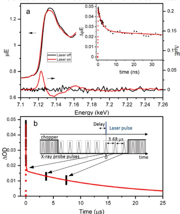
Figure 4. Fe K-Edge XTA a.) spectra and corresponding difference spectra for  $\text{NH}_2\text{-MIL-125(Ti,Fe)}$ . Inset: Kinetics monitored at 7.123 keV and b.) extended kinetics associated with synchronized and subsequent two X-ray probe pulses. Inset: schematic representation of XTA timing structure
