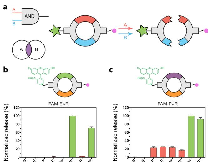
**Fig. 4** (a) Boolean AND-responsiveness is achieved through inclusion of two degradable moieties in parallel between gel (pink circle) and small molecule (green star). FAM is selectively released from gels for conditions involving (b) enzyme AND reductant, or (c) light AND reductant. X-axis labels indicating treatment conditions, release normalization criteria, histogram bar color, and error bar format match that described in Fig. 2.
