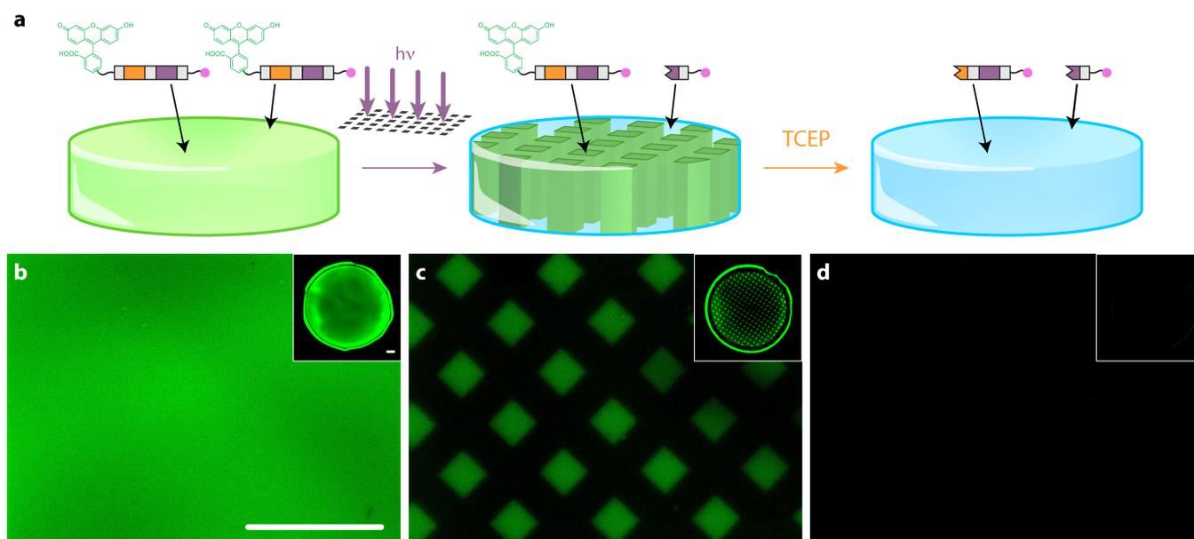
**Fig. 5** (a) Gels containing FAM-RVP exhibit sequentially triggered release in response to masked light followed by reductive treatment. Fluorescent images of gels (b) prior to treatment (N), after (c) exposure to photomasked light (P), and (d) successive incubation with TCEP (R). Insets depict full hydrogel imaged on a Typhoon gel scanner. Scale bars = 1 mm.
