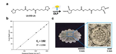
Fig. 2 (a) Photopolymerisation reaction of LA-EG-LA for the formation of a polymer network during the DLP printing process. (b) Jacobs working curves of LA-EG-LA with an LED at 405 nm. (c) 3D printed flower printed with a layer thickness of 100  $\mu$ m and a light intensity of 55 mW cm<sup>-2</sup>, light microscope image showing the highly detailed centre of the 3D printed flower.
