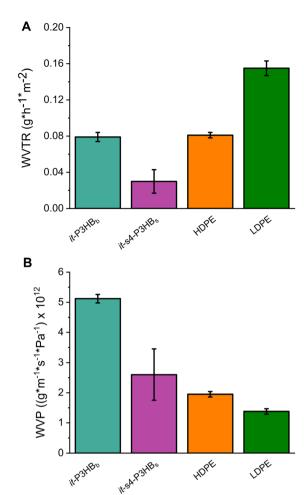
Fig. 6 WVTR (A) and WVP (B) of it-P3HB<sub>b</sub>, it-s4-P3HB ( $M_n = 152 \text{ kg mol}^{-1}$ , D = 1.22), and commodity plastics.
