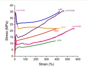
Fig. 4 Stress-strain curve overlays of it-s4-P3HB, ir-s4-P3HB, and srs4-P3HB with commodity plastics, including it-PP (blue), HDPE (orange), PBAT (red), and LDPE (green). Strain rate: 5.0 mm min<sup>-1</sup>, ambient temperature.
