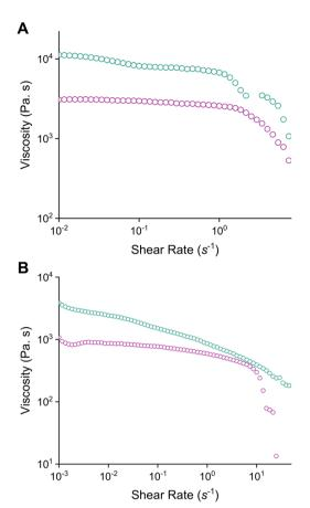
Fig. 5 Rheological properties of star-shaped P3HB (magenta) and linear P3HB (cyan curves): (A) ir-s4-P3HB (magenta) and ir-l-P3HB (cyan) overlays of rotational shear rheology curves; (B) sr-s4-P3HB (magenta) and sr-l-P3HB (cyan) overlays of rotational shear rheology curves.
