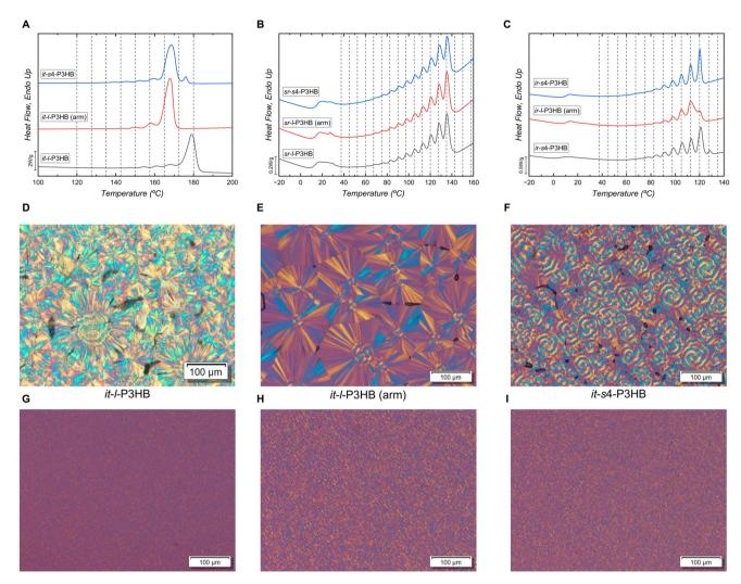
Fig. 2 Final DSC heating scans after SSA thermal fractionation (A–C) and PLOM micrographs (D–I) of it-P3HB (it-s4-P3HB, it-l-P3HB, and it-l-P3HB (arm)) and sr-P3HB (sr-s4-P3HB, sr-l-P3HB, and sr-l-P3HB (arm)). The (arm) denotes the lower molar mass linear P3HB with a chain length equivalent to one arm of star-shaped P3HB.
