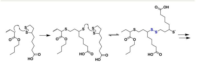
**Scheme 1** Copolymerisation of lipoic acid with n-butyl acrylate by radical ring-opening polymerisation. Two sequential additions of lipoic acid to the polymer forms a disulfide bond within the chain.
