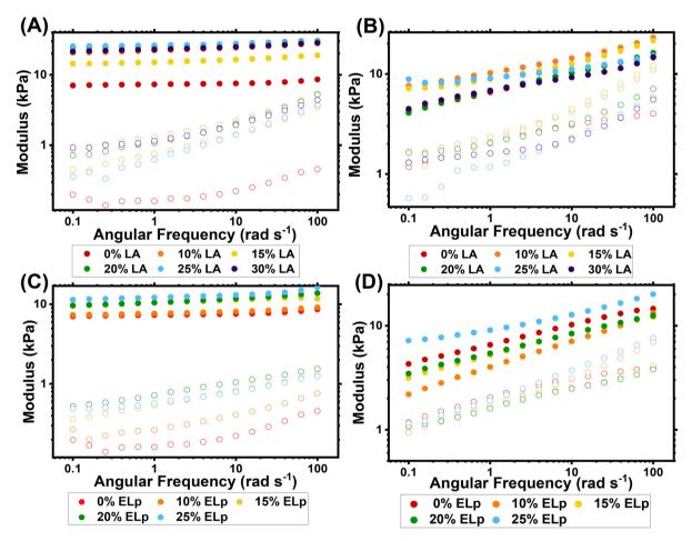
Fig. 1 Oscillatory rheology frequency sweep of (A and B) PBA-LA and (C and D) PBA-ELp gels synthesised by FRP (A and C) and RAFT (B and D). Closed symbols represent storage modulus (G') open symbols represent loss modulus (G'').
