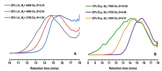
Fig. 2 GPC traces of the degraded gel fragments for (A) PBA-LA gels and (B) PBA-ELp gels synthesised by RAFT polymerisation.
