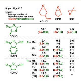
Fig. 3 Comparison of the  $M_n$  values and the average number of monomer units per block of the copolymers obtained by the copolymerization of oxiranes and cyclic hemiacetal esters ([oxirane]<sub>0</sub> = 0.75 M, [cyclic hemiacetal ester]<sub>0</sub> = 0.75 M,  $[B(C_6F_5)_3]_0$  = 1.0 or 3.0 mM), in dichloromethane at -78 °C. Ref. 12 and 13 for the DOLO and ROPT data, respectively (except for the DOLO-CPO copolymer [unpublished data]).
