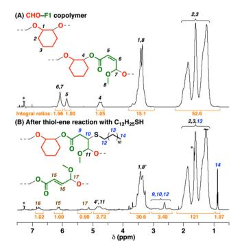
Fig. 6 <sup>1</sup>H NMR spectra of (A) CHO-F1 copolymer (obtained under similar conditions to those for entry 1 in Table 3; the average number of CHO/F1 units per block = 6.6/1.0) and (B) the product obtained by the thiol-ene reaction of the copolymer ([double bonds in copolymer] $_0$  =  $0.062 \text{ M}, [C_{12}H_{25}SH]_0 = 0.31 \text{ M}, [AIBN]_0 = 0.031 \text{ M}, in toluene at 80 °C,$ 24 h). See Fig. S22† for the MWD curves. \* CHCl<sub>3</sub> or water.
