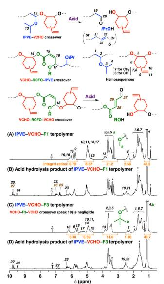
Fig. 5 <sup>1</sup>H NMR spectra of (A) IPVE-VCHO-F1 terpolymer (entry 1 in Table 3; Fig. 4A), (B) its acid hydrolysis product (purple curve in Fig. 4A), (C) IPVE-VCHO-F3 terpolymer (entry 3 in Table 3; Fig. 4B), and (D) its acid hydrolysis product (purple curve in Fig. 4B). In CDCl3 at 30 °C. \* CHClz, water, 1,2-dimethoxyethane, etc.
