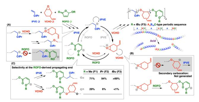
Scheme 5 Cationic terpolymerization of IPVE, VCHO, and ROFO: Propagation reactions at (A) VE-, (B) VCHO, and (C) ROFO-derived propagating ends.
