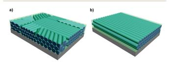
**Fig. 9** 2D hexagonal ordered porous material with (a) alignment defects and (b) uniform parallel orientation to the substrate. Reproduced from ref. 137 with permission from ACS, copyright 2025.
