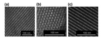
Fig. 12 TFM images of carbon films with well-ordered hexagonal structure (a-c). Reproduced from ref. 114 with permission from Elsevier, copyright 2025.
