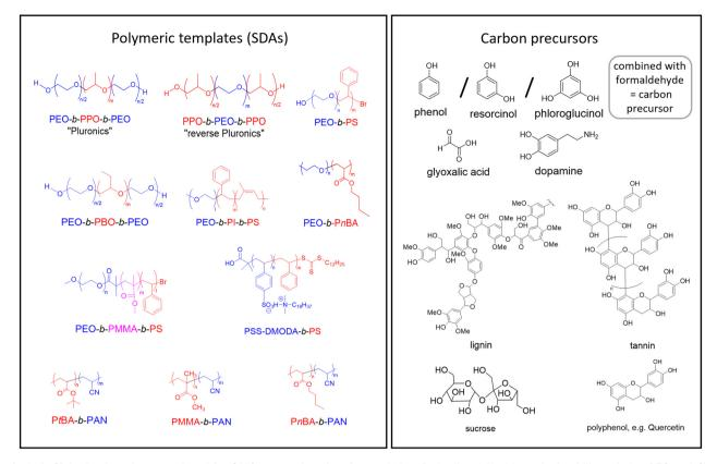
Fig. 1 Left: SDAs that have been employed for OMC preparation via soft-templating. Red = lipophilic, blue = hydrophilic moieties. PEO: poly(ethylene oxide), PPO: poly(propylene oxide), PS: polystyrene, PEA: poly(ethylene adipate), PSS-DMODA: poly(N,N-dimethyl-n-octadecylammonium p-styrenesulfonate), PBA: poly(n-butyl acrylate), PtBA: poly(tert-butyl acrylate), PAN: polyacrylonitrile, PMMA: poly(methyl methacrylate), PI: polyisoprene. Right: Frequently applied carbon precursors.
