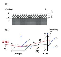
Fig. 10 General GI-SAXS setup: (a) medium 1 = vacuum; medium 2 = mesostructured thin film with thickness d; medium 3 = substrate with infinite thickness. (b)  $\alpha_i = \text{incident}$  angle;  $\alpha_f$  and  $2\theta_f = \text{exit}$  angles of the X-ray beam.  $k_i$  and  $k_f = \text{wave}$  vector of the incident and scattered X-ray beams.  $q_x$ ,  $q_y$ , and  $q_z = \text{components}$  of the scattering vector q. Reproduced from ref. 142 with permission from ACS, copyright 2025.
