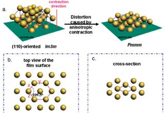
**Fig. 8** Illustration of (a) structural transformation of the OMC from *Im3m* to *Fmmm* symmetry during carbonization; distorted lattice from (b) the top and (c) cross-section. Reproduced from ref. 25 with permission from ACS, copyright 2025.
