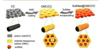
Fig. 15 Metal catalysts intended for HFR incorporated into OMCcoated carbon cloth. Reproduced from ref. 161 with permission from ACS, copyright 2025.
