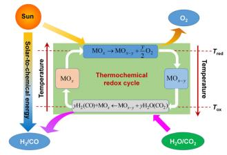
Fig. 1 Principle of two-step thermochemical cycling for solar fuel production based on ceria-based redox materials. Reproduced with permission<sup>11</sup> Copyright 2023, Elsevier
