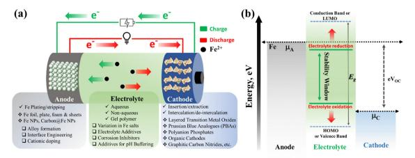
Fig. 2 (a) A detailed schematic of materials required for the anode, cathode, and electrolyte, including the charge-discharge mechanism. (b) Energy diagram showing different energy states of the anode, cathode, and electrolyte together with the stability window for rechargeable Fe-ion batteries.
