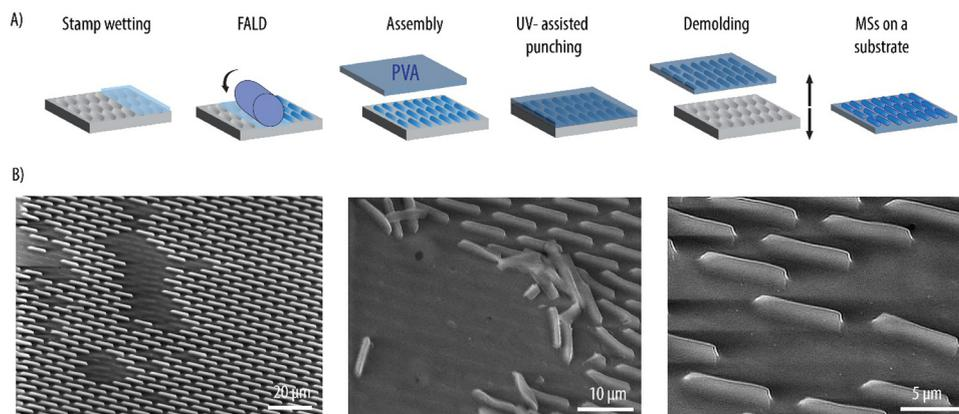
**Fig. 2** (A) Schematic illustration of force assisted liquid distribution (FALD) and UV-assisted punching processes employed to obtain rod-like microgel shapes (MSs). (B) Scanning electron microscopy micrographs of rod-like MSs at different magnifications obtained on a polyvinyl alcohol (PVA) substrate after UV-assisted punching.
