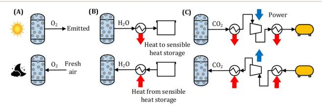
Fig. 2 Gas storage options for (A) redox, (B) hydroxide, and (C) carbonate reactions.
