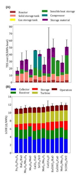
Fig. 6 (A) TES cost and (B) LCOE of the top twelve performing reactions selected based on LCOE. The error bars represent the LCOE and TES costs corresponding to halving and doubling the material price.
