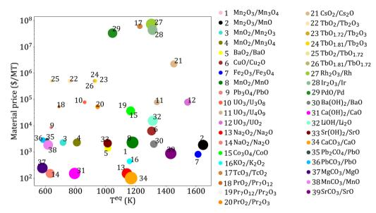
Fig. 5 Key parameters for reactions obtained after applying thermodynamic criteria. Each bubble represents a candidate reaction, and its size represents reaction enthalpy.
