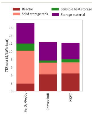
Fig. 9 A comparison of TES cost of Fe<sub>2</sub>O<sub>3</sub>/Fe<sub>3</sub>O<sub>4</sub> system with the target TES cost obtained by convex hull and NKVT approach.
