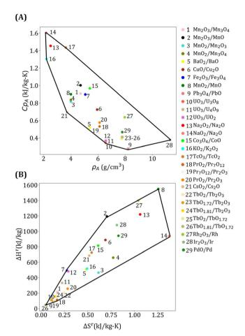
Fig. 4 Data and convex hull of (A) heat capacity and density of A, and (B) reaction enthalpy and entropy for reaction set N.
