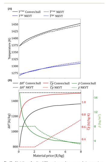
Fig. 11 Variation of optimal (A) receiver and power-cycle temperature, and (B) reaction enthalpy, average heat capacity, and average density of solid materials with price.
