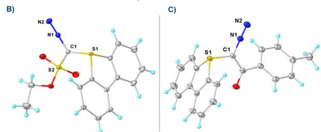
**Scheme 2** (A) Synthesis of  $\alpha$ -diazosulfonium salts; (B) and (C) molecular structures in the solid state of compounds **1a** and **1c**, respectively. Anisotropic displacements shown at the 50% probability level. Triflate anions and solvent molecules omitted for clarity. Selected bond lengths [Å]: **1a**: S1–C1, 1.728(1); C1–N1, 1.333(1); N1–N2, 1.113(1); **1c**: S1–C1, 1.742(2); C1–N1, 1.339(2); N1–N2, 1.117(2).
