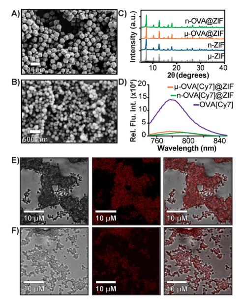
Fig. 1 Characterization of OVA@ZIF. (A) SEM images of  $\mu$ -OVA@ZIF and (B) n-OVA@ZIF. (C) PXRD diffractogram of OVA@ZIF composites. (D) Encapsulation efficiency of  $\mu$ -OVA[Cy7]@ZIF and n-OVA[Cy7]@ZIF as measured by Cy7 fluorescence in the supernatant ( $\lambda_{ex}=756$  nm and  $\lambda_{em}=779$  nm). (E) CLSM images of  $\mu$ -OVA[Cy7]@ZIF and (F) n-OVA[Cy7]@ZIF. Brightfield images are shown on the left, fluorescent in the middle, and merged channels on the right.
