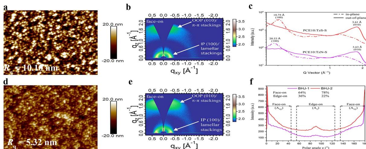
**Fig. 4** AFM images and 2D GIWAX patterns of PCE10:TzN-S (a and b) and PCE10:TzS-S (d and e) blend films along with the corresponding 1D line-cut profiles (c). Pole figure plot (f) extracted from the IP (100) lamellar scattering, each of BHJ-1 (PCE10:TzN-S) and BHJ-2 (PCE10:TzS-S) film, where polar angle ( $\chi$ ) range<sup>43</sup> is defined corresponding to the face-on ( $A_{xy}$ ) and edge-on ( $A_z$ ) crystallites.
