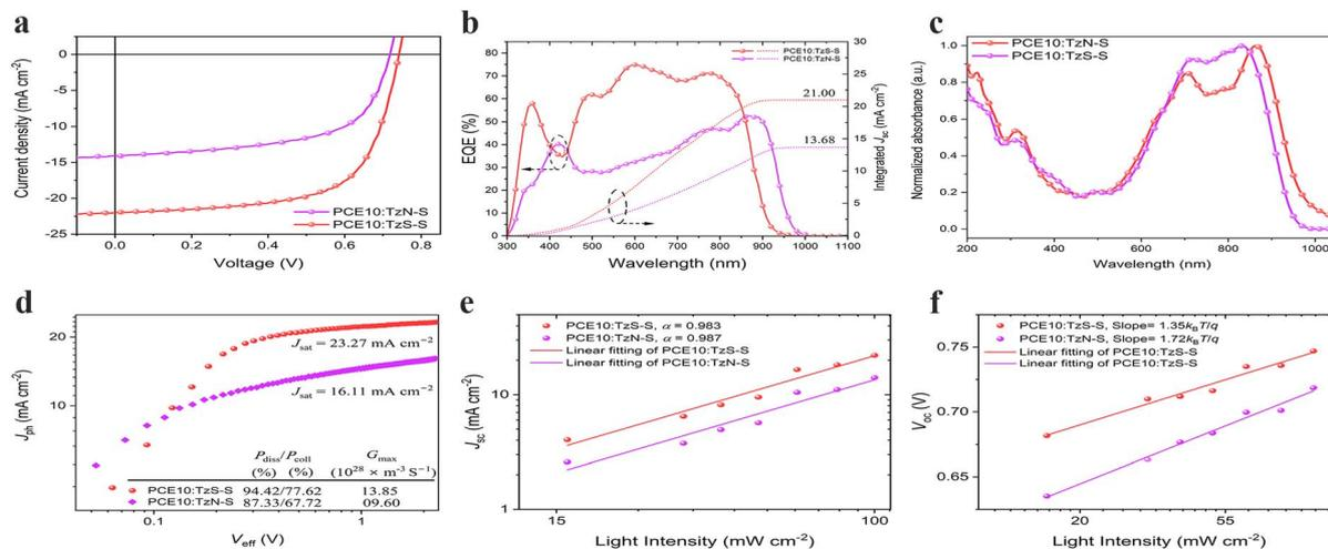
Fig. 3 (a)  $J$ - $V$  curves and (b) corresponding EQE spectra of the optimal PCE10: acceptor based OSC devices. (c) Normalized UV-vis-NIR absorption spectra of the blend films under study. (d)  $J_{ph}$ - $V_{eff}$  characteristics, (e) light intensity dependence of  $J_{sc}$  showing negligible bimolecular recombination, and (f) variation of  $V_{oc}$  with light intensity for PCE10:acceptor based fabricated devices.
