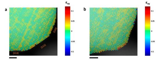
Fig. 5 Strain analysis of a PtCu<sub>3</sub> nanoparticle. Shear strain ( $\varepsilon_{xy}$ ) map (a) before and (b) after electrochemical activation. 60 Open access, 2019.
