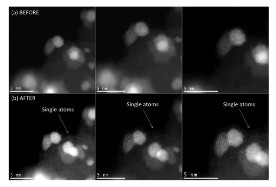
Fig. 7 IL-STEM images of  $Pt-SnO_2/C$  nanoparticles (a) before and (b) after 1000 electrochemical cycles from 0.05-9.8 V (vs. RHE) at different magnifications. Single atoms appear after degradation and are shown to not move from beam exposure. Reprinted with permission from J. Phys. Chem. C, 2018, 122(18), 10050-10058.96 Copyright 2018, American Chemical Society.
