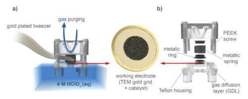
Fig. 8 An illustration of the modified floating electrode (MFE) setup. 97 Open access, 2020.
