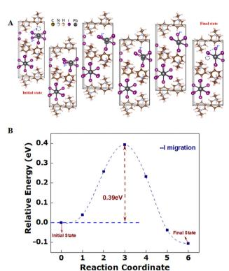
Fig. 4 Halide migration in PrPyrPbI<sub>3</sub>: (A) migration pathway, dotted blue lines show the vacancy migration and black dashed circles represent the vacancies. (B) Energy barrier corresponding to the ion migration barrier.
