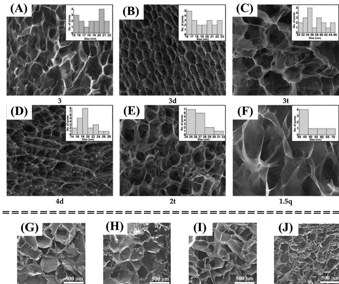
Fig. 7 The porosity is increased with increasing the water quantity in the hydrogel composition from 97.88% to 99.30% reported by Craciun *et al.* (2022) (A)–(F).<sup>127</sup> The variation of pore size is increased with the degree of substitution (DS) reported by Fengjiao Zhang *et al.* (2023)<sup>156</sup> (G)–(J). Figures are reproduced from open access articles.
