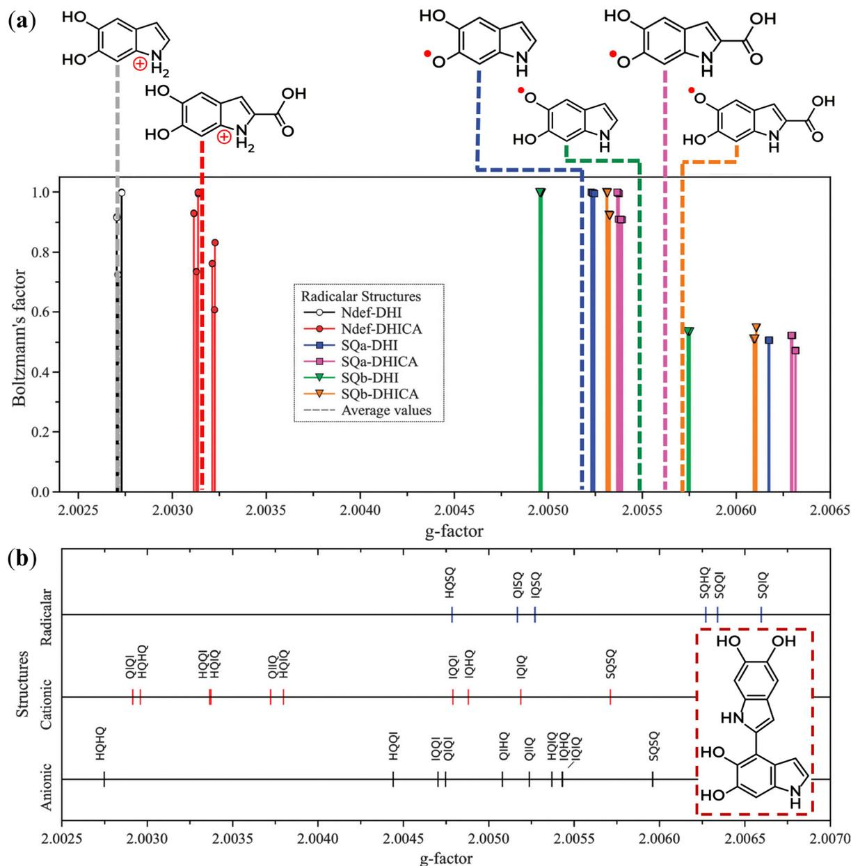
**Fig. 8** Distribution of the theoretical  $g$ -values from eumelanin moieties that are: (a) radical monomers and (b) homo- and hetero-dimers. Compatible behavior was obtained for anionic and cationic monomers. The inset in (b) represents an example of a homo-dimer. Reproduced from A. Batagin-Neto *et al.* (2015)<sup>77</sup> with permission from the PCCP Owner Societies.
