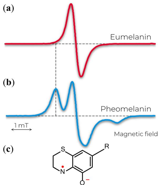
**Fig. 3** X-band EPR spectra of (a) eumelanin and (b) pheomelanin. The extra feature in *b* is attributed to the nitrogen hyperfine coupling of (c) *o*-semiquinonimine. (a) Adapted with permission from J.V. Paulin *et al.* (2019).<sup>78</sup> Copyright© 2019, American Chemical Society. (b) Adapted with permission from A. Zadlo *et al.* (2018).<sup>79</sup> Copyright© 2018, John Wiley & Sons.
