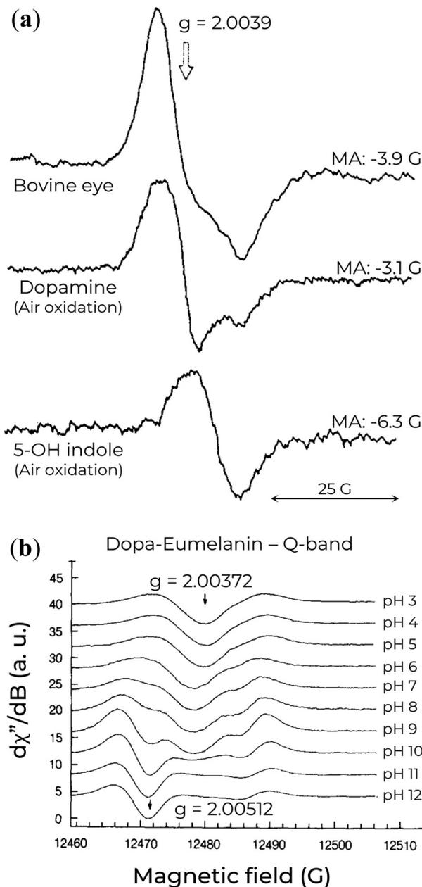
Fig. 9 (a) Q-band EPR spectra of eumelanin and eumelanin-inspired materials. MA indicates the modulation amplitude. Reprinted with permission from F.J. Grady and D.C. Borg (1968).<sup>129</sup> Copyright © 1968, American Chemical Society. (b) Variation of Q-band EPR signal of Dopa-Eumelanin as a function of pH. Reprinted with permission from M. Pasenkiewicz-Gierula and R.C. Sealy (1986).<sup>99</sup> Copyright © 1986, Elsevier B.V.
