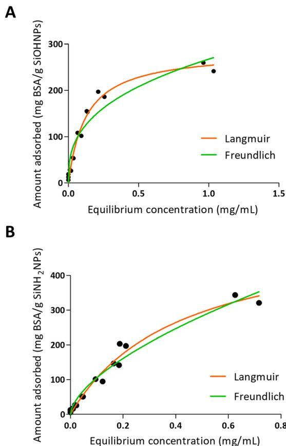
Fig. 3 Adsorption isotherms of BSA over SiOHNPs (A) and SiNH<sub>2</sub>NPs (B) with representation of Langmuir and Freundlich curves in orange and green, respectively.
