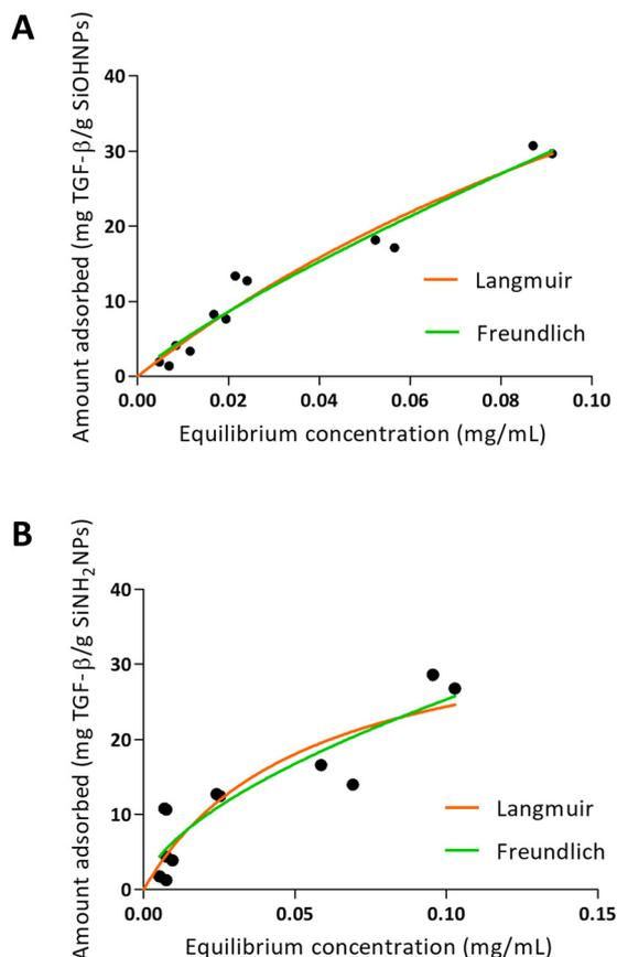
Fig. 5 Adsorption isotherms of TGF- $\beta$  over SiOHNP (A) and SiNH<sub>2</sub>NP (B) with representation of Langmuir and Freundlich curves in orange and green, respectively.
