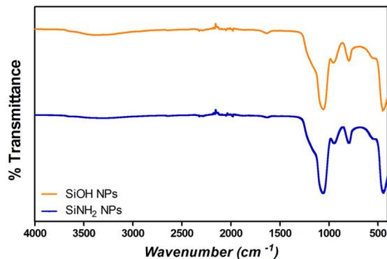
Fig. 2 FTIR analysis of SiOH NPs (orange) and SiNH<sub>2</sub> NPs (blue).
