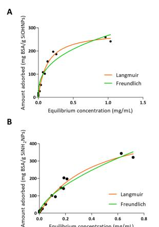
Fig. 3 Adsorption isotherms of BSA over SiOHNPs (A) and SiNH<sub>2</sub>NPs (B) with representation of Langmuir and Freundlich curves in orange and green, respectively
