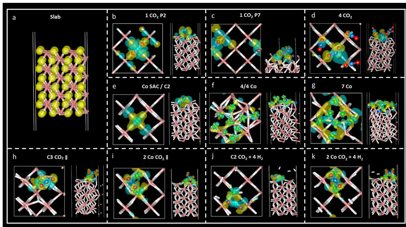
**Fig. 5** Charge density difference maps ( $\rho_{\text{system}} - \rho_{\text{slab}} - \rho_{\text{Co}} - \rho_{\text{gas}}$ ) for the most stable structures (a–k) with the isosurface value of 0.005e. The yellow region represents charge density accumulation, while the blue region represents charge depletion.
