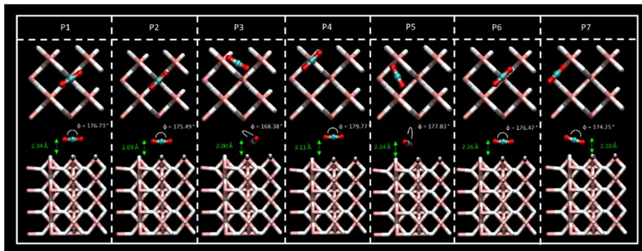
Fig. 2 Top- and side-view of the CO<sub>2</sub> adsorption structures for the P1–P7 sites, where CO<sub>2</sub> bending angles and CO<sub>2</sub>–slab distances are shown. Atom colour code: (white) hydrogen, (pink) magnesium, (red) oxygen, (blue) carbon.
