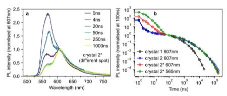
Fig. 5 Anomalous photoluminescence behaviour of rubrene crystals. (a) Time-gated PL spectra, normalised at 607 nm, for crystal 2\*, a different spot on the surface of crystal 2 that exhibited similar PL behaviour to that reported in ref. 10. (b) Time-dependence of the PL intensity from crystals 1, 2 and 2\* at various detection wavelengths, normalised at 100 ns.
