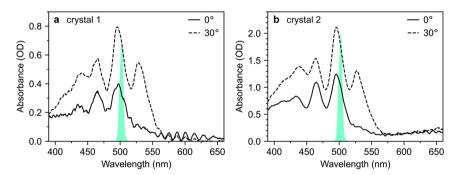
Fig. 3 Absorption spectra of rubrene single crystals. (a and b) Absorption spectra of crystals 1 and 2, respectively, at both 0° and 30° degree incidence angles. The spectra of the excitation pulses are also shown in cyan.
