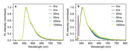
Fig. 12 TRPL of polycrystalline rubrene. (a and b) Time-gated photoluminescence spectra of a polycrystalline rubrene film following excitation at 500 nm (a) and 532 nm (b).
