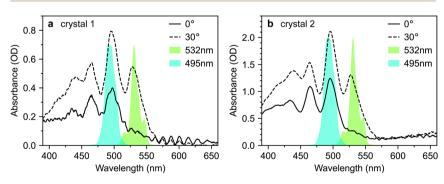
Fig. 7 Selective excitation of rubrene single crystals. (a and b) Absorption spectra of rubrene single crystals 1 and 2 at incidence angles of 0° and 30°, reproduced from Fig. 3. The 495 nm and 532 nm pump spectra used in the transient absorption experiments presented in this paper are shown. The two pump wavelengths target the 0-1 and 0-0 vibronic transitions, respectively.
