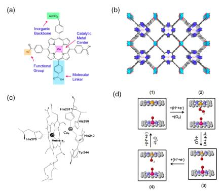
Fig. 5 (a) and (b) Coordination entity for constructing  $Al_2(OH)_2TCPP-Co$  MOF. Adapted from ref. 55 with permission. (c) Cytochrome-C oxidase enzyme. Adapted from ref. 58 with permission. (d) Illustration of the bio-mimic prototype catalyst capable of circumventing the scaling relations.
