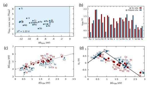
Fig. 10 (a) Stability of single metal atoms in  $SnO_2$  in terms of dissolution potential vs. formation energies, (b) theoretical overpotentials for the ORR with different doped-metals in  $SnO_2$ , (c) scaling relationship between ORR intermediates, and (d) activity volcano plot for the 4e-ORR. Data adapted from ref. 92 with permission.
