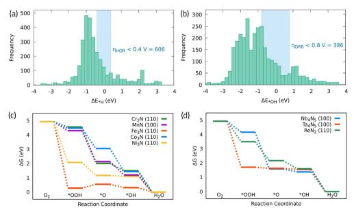
Fig. 8 (a) and (b) Distribution of \*H and \*OH adsorption free energies across different TMNs studied in ref. 74, respectively. (c) Calculated free energy diagram for ORR on different first row (d) and second/third row TMN surfaces. The corresponding data and structures can be found in the ESI.†
