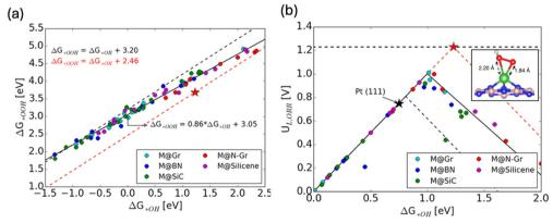
Fig. 4 (a) Scaling relationship for the chemisorption energies of OH\* and OOH\* for various SACs. (b) Activity volcano plots for SACs (solid black), metal (111) (dashed black) and ideal catalyst (dashed red). Inset shows the bidentate adsorption stabilizes OOH\* intermediate and results in overall improved activity. Copyright with permission from ref. 42.
