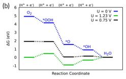
Fig. 2 (a) Free energy diagram for oxygen reduction on ideal catalyst for two- and four-electron oxygen reduction. (b) Free energy diagram for oxygen reduction on Pt(111) associative mechanism. Data for Pt(111) are adapted from ref. 15
