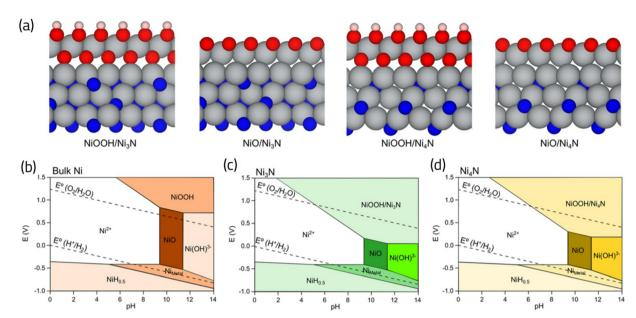
Fig. 9 (a) Atomic structures showing formation of oxide (NiOOH and NiO) layers on  $Ni_3N$  and  $Ni_4N$  nitride surfaces. (b)–(d) Constructed Pourbiax diagrams for bulk Ni,  $Ni_3N$  and  $Ni_4N$ , respectively. The extension of NiOOH phase is evident in (b) and (c) compared to bulk Ni, highlighting the propensity of nitride surfaces to develop oxide films under the relevant pH and potentials of ORR. Adapted from ref. 80 with permission.
