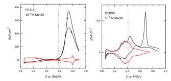
Fig. 7 Voltammetric profiles for the methanol oxidation reaction in 0.1 M HClO $_4$  (black curves) on Pt(111) and Pt(100) electrodes. The red curves show the profiles obtained in the absence of methanol and the vertical dashed lines represent the onset of OH adsorption on these surfaces. Scan rate: 50 mV s $^{-1}$ .
