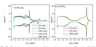
Fig. 2 Evolution upon cycling of the voltammetric profiles of a Pt(111) electrode in 0.5 M  $\rm H_2SO_4$  and 0.1 M  $\rm HClO_4$  with different levels of impurities. Scan rate: 50 mV s<sup>-1</sup>.
