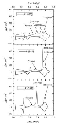
CO stripping profiles for different stepped and kinked surfaces in 0.1 M NaOH. The arrows indicate the origin of the different peaks. Scan rate:  $50 \text{ mV s}^{-1}$
