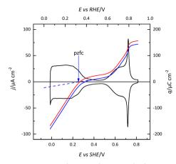
Fig. 5 Voltammetric profile (black line) of the Pt(111) electrode in  $0.1~\rm M$  HClO $_4$  and integration curves using the CO displaced charge displaced at  $0.1~\rm V$  before (red line) and after (blue line) correction for the residual charge of CO CO-covered electrode. The blue dashed line shows the extrapolation of the straight region to determine the pzfc.
