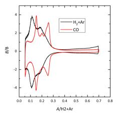
Fig. 4 Voltammetric profile for the Pt(110) electrode in 0.1 M HClO<sub>4</sub> cooled down in different atmospheres. Scan rate:  $50 \text{ mV s}^{-1}$
