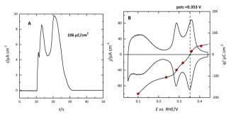
Fig. 3  $\,$  (A) CO displaced charge at 0.24 V for the Pt(311) electrode in 0.1 M  $\,$ HClO<sub>4</sub>. (B) Voltammetric profile (left axis) and total charge curve (right axis) for the Pt(311) electrode in 0.1 M HClO<sub>4</sub>. The red points indicate the displaced charge used as integration constants for the charge curve. Scan rate:  $50 \text{ mV s}^{-2}$
