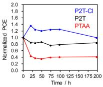
Fig. 6 Long-term stability of P2T, P2T-Cl and PTAA based PSCs. The PSCs were stored in an environmental test chamber at 30 °C and relative humidity of 60% in darkness.
