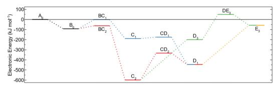
Fig. 3 Energy profile for TMA adsorption and decomposition on amino terminated AlN. The black step ( $A_0$  to  $B_0$ ) is initial adsorption of TMA. The blue path (Bo via C1 to D1) is methyl protonation followed by reductive elimination and red (Bo via C2 to D1) is reductive elimination followed by methyl protonation. The yellow path ( $D_1$  to  $E_3$ ) is surface oxidation, and the green ( $C_2$  via  $D_3$  to  $E_3$ ) is surface oxidation followed by methyl protonation.
