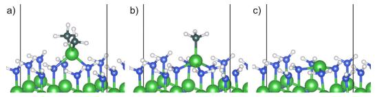
Fig. 2 Geometries for (a) DMA fragment after methyl protonation ( $C_1$ ), (b) MMA fragment after reductive elimination ( $C_2$ ) and (c) aluminum adatom after methyl protonation followed by reductive elimination ( $D_1$ ).
