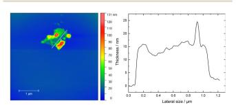
Fig. 4 AFM image and the corresponding height profile plot of exfoliated NiGa<sub>2</sub>S<sub>4</sub>
