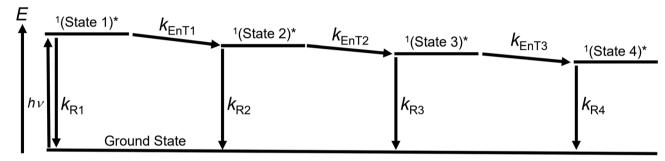
Scheme 1 Proposed kinetic models for emission processes from multiple aggregate states and related processes in (0Ph-B-BODIPY)<sub>m</sub>
