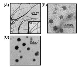
Fig. 2 TEM images of (A)  $(OPh-B-BODIPY)_m$ , (B)  $(1Ph-B-BODIPY)_m$ , and (C)  $(2Ph-B-BODIPY)_m$  prepared in  $H_2O/THF = 99/1$  (v/v).
