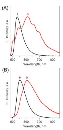
Fig. 5 Fluorescence spectra of (A) (a) OPh-B-BODIPY (monomer: black) in THF and (b)  $(OPh-B-BODIPY)_m$  in  $H_2O/THF = 99/1$  (v/v) (red) and (B) (a) 1Ph-B-BODIPY (monomer: black) in THF and (b) (1Ph-B-BODIPY)<sub>m</sub> in  $H_2O/THF = 99/1 \text{ (v/v) (red)}, \lambda_{ex}$ : 470 nm.
