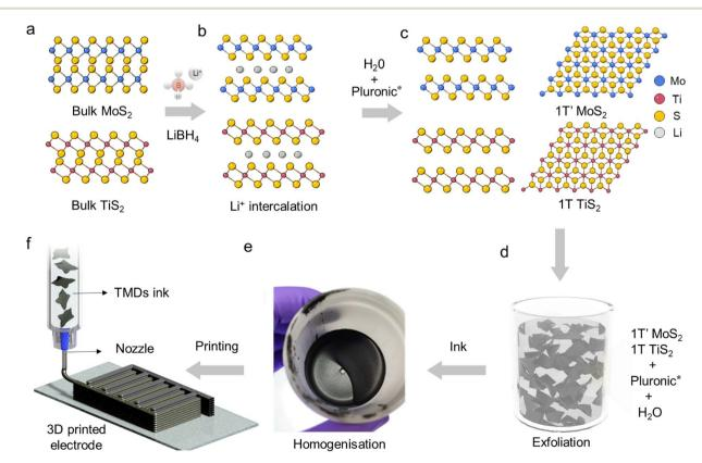
Scheme 1 Schematic representation of the synthesis process, exfoliation mechanism and 3D printing of 1T'/1T MoS<sub>2</sub>/TiS<sub>2</sub> inks. (a) Atomic structures of bulk MoS<sub>2</sub> and TiS<sub>2</sub> and (b) atomic lattices of lithiated MoS<sub>2</sub> and TiS<sub>2</sub>. (c) and (d) Pluronic-water exfoliation process of MoS<sub>2</sub> and TiS<sub>2</sub>. (e) Homogenization of 1T'/1T MoS<sub>2</sub>/TiS<sub>2</sub> inks and (f) extrusion of the corresponding inks through a nozzle.
