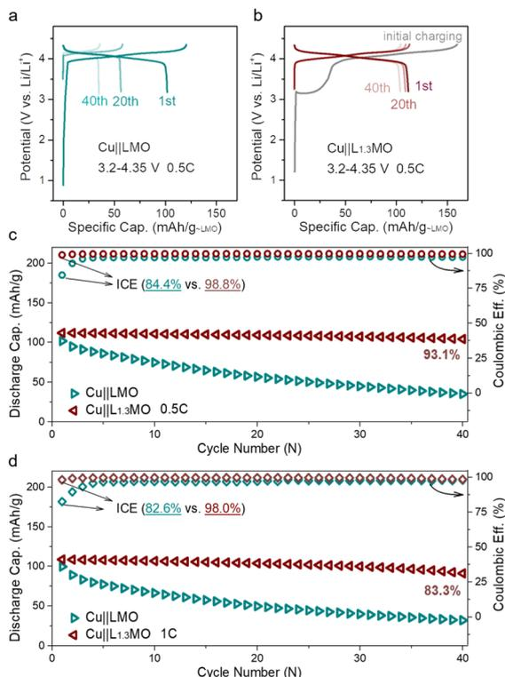
Fig. 3 Charge–discharge curves of (a)  $Cu||LMO$  and (b)  $Cu||L_{1.3}MO$  anode-free coin cells, and (c) corresponding cycling performance and CE of (a) and (b) at 0.5C discharge rate. (d) Cycling performance and CE of  $Cu||LMO$  (Fig. S19a<sup>†</sup>) and  $Cu||L_{1.3}MO$  (Fig. S19b<sup>†</sup>) at 1C discharge rate. ( $L_{1.3}MO$  cathodes were prepared *via* the electrochemical pre-lithiation method).
