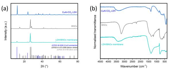
Fig. 1 (a) pXRD patterns and (b) FT-IR spectra of CuAl-CO<sub>3</sub> LDHs (blue), BNOx (grey) and LDH/BNOx nanocomposite (turquoise). pXRD reference patterns are provided for CuAl hydrotalcite, boron nitride and boric acid.
