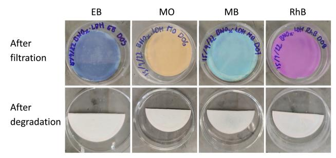
Fig. 8 Pictures of membranes before (top) and after (bottom) photodegradation using 10 μL H<sub>2</sub>O<sub>2</sub> (30% w/w) and a 5 W COB LED.
