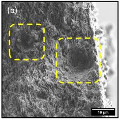
Fig. 9 SEM images depicting (a) exfoliation of membrane and (b) formation of micro-bubble shaped cavities in membrane during photo-degradation process.
