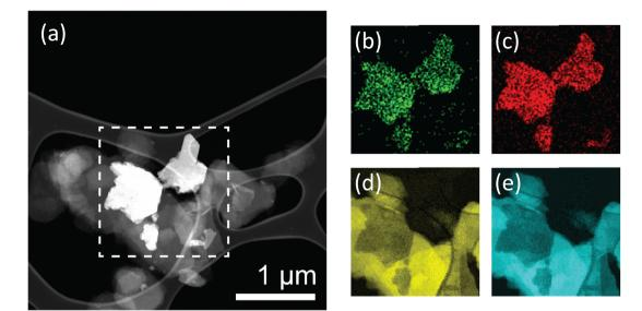
Fig. 3 HAADF-STEM image (a) of LDH/BNOx nanocomposite. Dashed box in (a) is area under analysis in (b) – (e). Elemental mapping of Al (b) and Cu (c) via EDX, and N (d) and B (e) via EELS. Scale bar in (b)-(e) is same as in (a).
