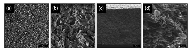
Fig. 2 (a and b) Top-view and (c and d) cross-sectional SEM images of LDH/BNOx membranes. Lower magnification images (a and c) show general uniformity of membranes, and higher magnification (b and d) shows finer membrane structure consisting of networks of nanosheets.
