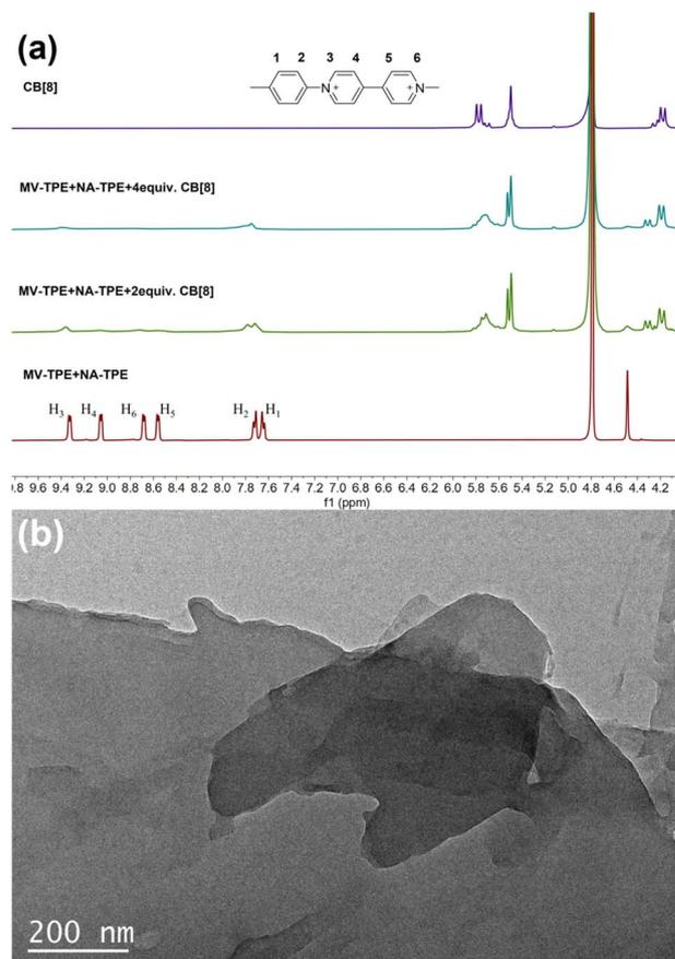
Fig. 2 (a) <sup>1</sup>H NMR (400 MHz, D<sub>2</sub>O, 298 K) spectra of MV-TPE + NA-TPE, MV-TPE + NA-TPE + 2 equiv. CB[8], MV-TPE + NA-TPE + 4 equiv. CB[8] and CB[8]. (b) TEM image of MV-TPE + NA-TPE + CB[8] (1 : 1 : 4, 2.0 × 10<sup>-5</sup> M).
