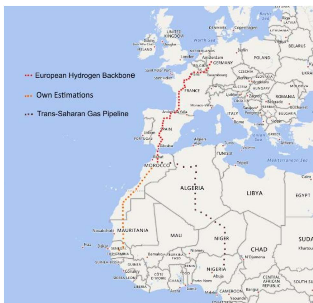
Fig. 1 Hydrogen supply chain. Red-colored route is possible corridor for German imports based on existing natural gas infrastructure (European Hydrogen Backbone). 28 The routes in Africa are estimated on the basis of our own calculations and the planned Trans-Saharan Gas Pipeline project.
