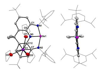
Fig. 3 Left: Solid-state structure of 4. Right: Side view of the anionic part of 4. The  $^t$ Bu and Dipp groups are simplified as wireframes and hydrogen atoms are omitted for clarity. Thermal ellipsoids are set at the 30% probability level. Selected bond lengths (Å) and angles (°): Ge1–N1 2.0578(18), Ge1–N2 2.1633(18), Ge1–N3 1.9039(19), C1–N1 1.372(3), C7–N2 1.359(3), C6–N3 1.388(3), C12–N3 1.384(3), C1–C6 1.414(3), C7–C12 1.428(3), N1–Ge1–N2 153.81(7), N1–Ge1–N3 78.23(7), N2–Ge1–N3 76.56(7).
