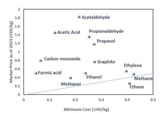
Fig. 3 Possible electrocatalytic  $CO_2$  reduction reaction products plotted as a function of minimum energy consumption per unit mass and market price as of 2023. The line represents the break-even point assuming no additional financial incentives.
