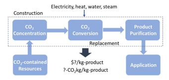
Fig. 4 Basic processes for a scaled-up electrocatalytic CO<sub>2</sub> reduction reaction: CO<sub>2</sub> purification, CO<sub>2</sub> conversion, and product purification.
