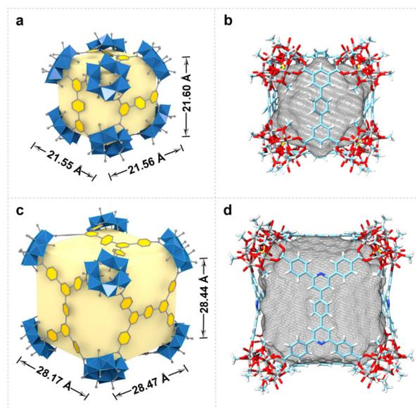
**Fig. 3** Crystal structures of **VMOC-4** (a and b) and **VMOC-6** (c and d). The left column highlights the overall size of each cubic cage and the arrangement of the ligands, while the right column shows the void spaces (gray mesh) calculated using the VOIDOO program.
