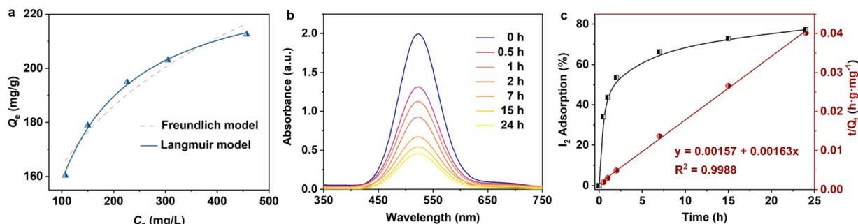
**Fig. 5** (a) Langmuir and Freundlich model fitting of the isotherm of iodine adsorption by **VMOC-6** in cyclohexane solution. (b) Time evolution of the UV-vis absorption spectra of cyclohexane solutions in the presence of **VMOC-6**. (c) The kinetics of the adsorption process of iodine on **VMOC-6** was plotted with the relative removal rate (%) of iodine (black line) and  $t/Q_e$  (red line) *versus* time.
