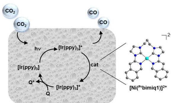
Fig. 1 Photocatalytic CO<sub>2</sub> reduction process by the [Ni(<sup>Pr</sup>bimiq1)]<sup>2+</sup> complex. Reprinted with permission from ref. 26. Copyright 2013 American Chemical Society.
