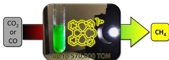
**Fig. 2** Photocatalytic reduction of CO<sub>2</sub>/CO to CH<sub>4</sub> by the Ni<sup>II</sup>-NHC-bipyridyl complex. Reprinted with permission from ref. 30. Copyright 2019 American Chemical Society.
