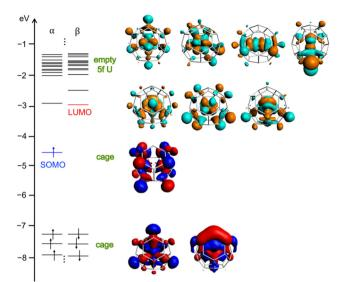
Fig. 3 Frontier molecular orbitals of U@C<sub>27</sub>B at PBE0/TZP level. SOMO and LUMO are essentially cage orbitals and all U-5f orbitals are empty.
