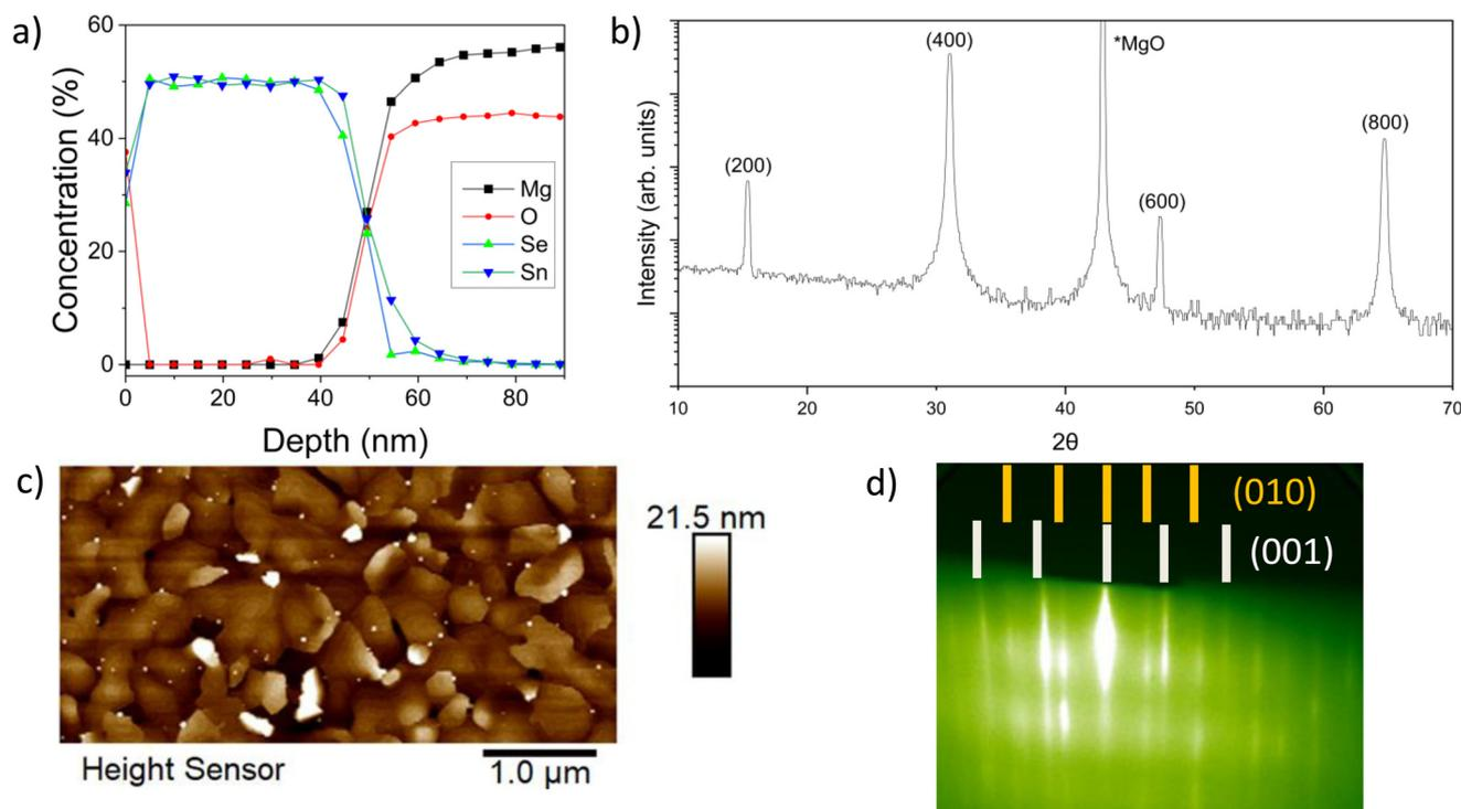
**Fig. 2** (a) XPS depth profile of a SnSe thin film deposited on MgO with 1 : 4 Sn : Se flux ratio at  $280 \pm 5$  °C for 83 minutes. (b) XRD of the film in 2a indicating (200) orientation out-of-plane, (c) AFM on the same film showing mixed orientation distribution in-plane, and (d) RHEED measurements of a SnSe film with multiple in-plane orientations taken post growth.
