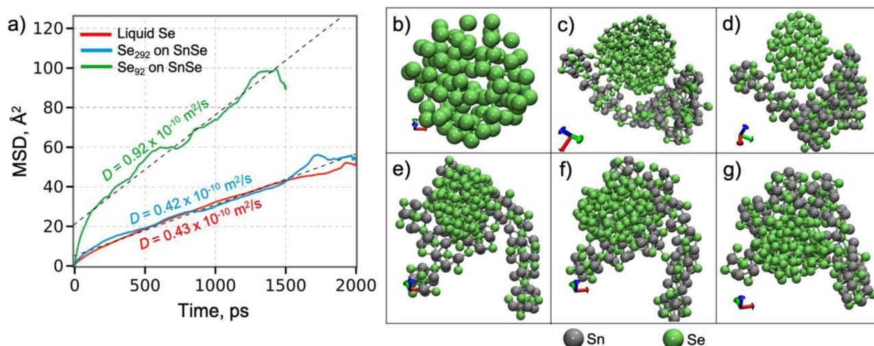
**Fig. 4** Diffusion of Se atoms in the Se cluster at 500 K. (a) The mean-square displacement as a function of time of Se atoms. Dashed lines are a linear regression of the MSD curves. (b) A free liquid Se cluster. (c) A  $\text{Se}_{292}$  cluster on the SnSe surface. (d) An edge-bound Se cluster. (e–g) A  $\text{Se}_{92}$  cluster on the SnSe surface at 96.5 ps, 289.6 ps and 407.5 ps, respectively.
