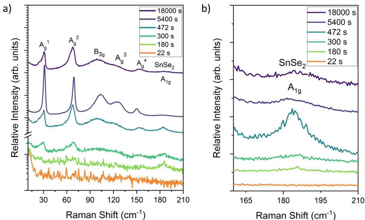
**Fig. 5** Raman spectra of  $Pnma$  SnSe thin films taken for different deposition times across (a) the full range of vibrational modes and (b) focused on the region indicating the SnSe<sub>2</sub>  $A_{1g}$  mode.
