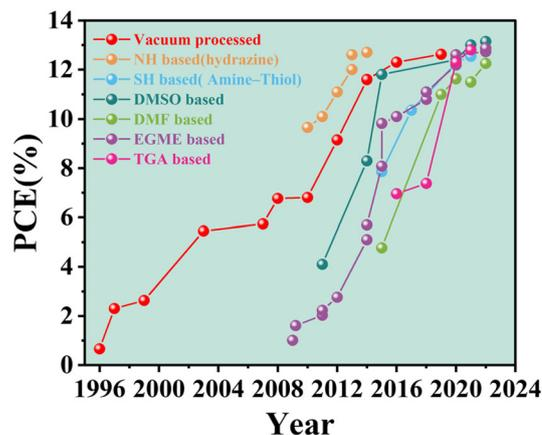
Fig. 1 The power conversion efficiency evolution of Cu<sub>2</sub>ZnSn(S,Se)<sub>4</sub> Solar Cells.
