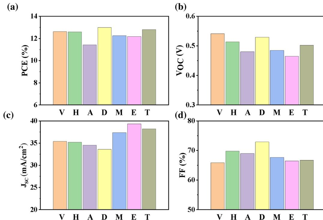
Fig. 10 (a–d) Experimental device performance values for efficiency,  $V_{oc}$ ,  $J_{sc}$ , and FF for champion vacuum<sup>25</sup> and solution-processed CZTSSe (H,<sup>30</sup> A,<sup>65</sup> D<sup>24</sup>, M,<sup>117</sup> E,<sup>120</sup> and T<sup>146</sup>) solar cells, respectively.
