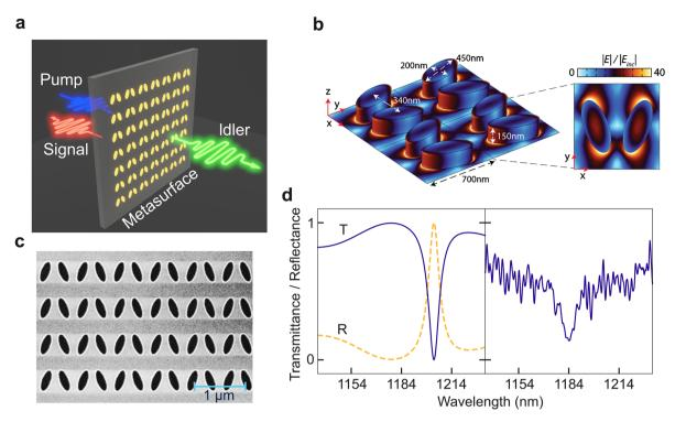
Fig. 1 (a) SPDC in a metasurface with the signal and idler photons emitted in opposite directions. (b) The shape and dimensions of the unit cell and the electric field distribution. (c) An SEM view of the metasurface. (d) Left: the calculated white-light transmission (blue) and reflection (orange) spectrum of the metasurface. Right: the measured transmission spectrum.
