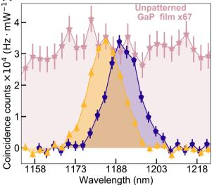
Fig. 4 Enhancement of photon pair generation. Coincidence counts rate per pump power for the metasurface (color) and an unpatterned 150 nm thick GaP film (grey stars). In the latter case, the measurement was made for a 400 nm film and the rate was reduced to account for the smaller thickness.
