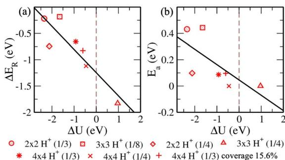
Fig. 8 (Color online) Variation of (a) reaction energy ( $\Delta E_R = E_{\text{final}} - E_{\text{initial}}$ ) and (b) activation energy ( $E_a$ ), of configurations with respect to the change in electrode potential ( $\Delta U = U_{1_{\text{initial}}} - U_{1_{\text{final}}}$ ) from initial to final.
