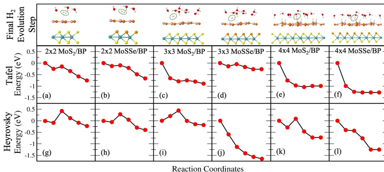
Fig. 4 (Color online) (a)–(f) Tafel reaction path (upper row) on MoS<sub>2</sub>/BP and MoSSe/BP vdW HTSs for  $2 \times 2$ ,  $3 \times 3$  and  $4 \times 4$  supercells. (g)–(l) Heyrovsky reaction path (lower row) on MoS<sub>2</sub>/BP and MoSSe/BP vdW HTSs for  $2 \times 2$ ,  $3 \times 3$  and  $4 \times 4$  supercells.
