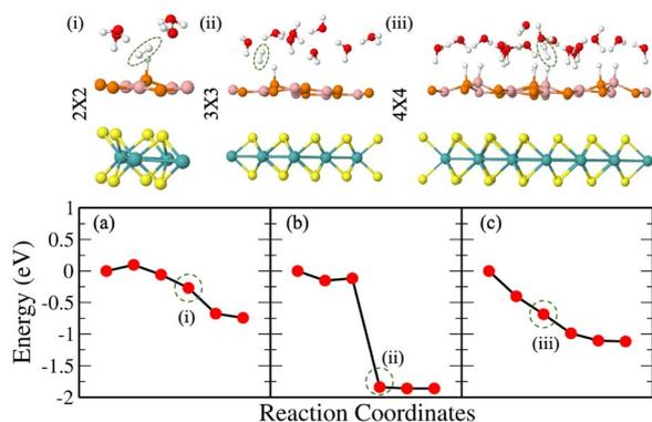
Fig. 6 (Color online) Heyrovsky reaction path for the  $\text{MoS}_2/\text{BP}$  vdW HTS with  $1/4\text{H}^+$  conc. in (a)  $2 \times 2$  supercell, (b)  $3 \times 3$  supercell and (c)  $4 \times 4$  supercell.
