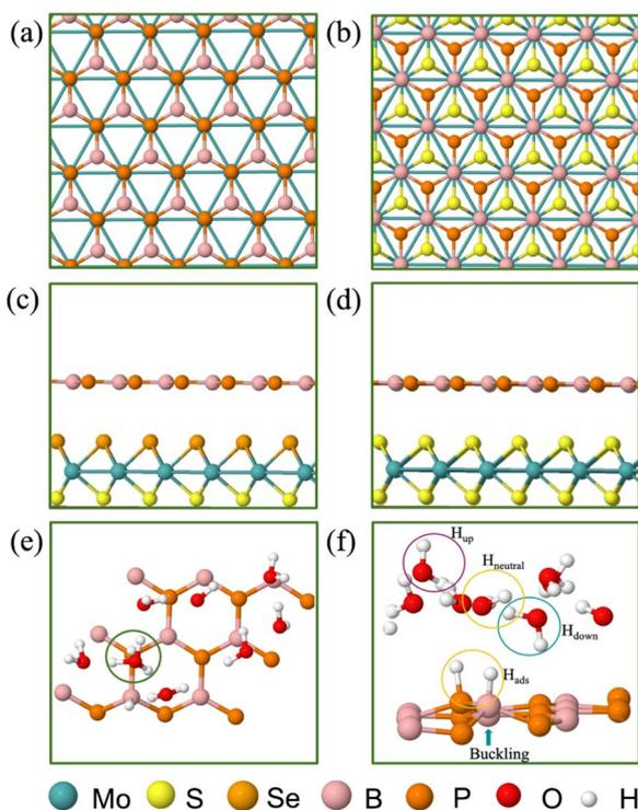
Fig. 2 (Color online) (a) and (b) Top view of MoS<sub>2</sub>/BP vdW HTS stacking configurations, (c) and (d) side view of minimum energy stacking configuration for MoS<sub>2</sub>/BP and MoSe/BP vdW HTSs, respectively, (e) 3 × 3 supercell of the BP monolayer schematic with 1/3H<sup>+</sup> conc. *i.e.*, 1H<sup>+</sup>/3H<sub>2</sub>O, and (f) water molecule orientations of H<sub>up</sub>, H<sub>down</sub> and H<sub>neutral</sub>. Buckling on BP can be observed at the H<sub>ads</sub> site.
