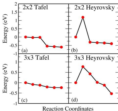
Fig. 3 (Color online)  $2 \times 2$  supercell of the BP monolayer showing (a) Tafel reaction path and (b) Heyrovsky reaction path. The  $3 \times 3$  supercell of the BP monolayer showing (c) Tafel reaction path and (d) Heyrovsky reaction path.
