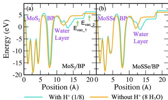
Fig. 7 (Color online) Electrostatic potential plot of (a) MoS<sub>2</sub>/BP and (b) MoSSe/BP vdW HTSs depicting the water layer with and without H<sup>+</sup> in 3 × 3 supercell (*i.e.*, 1/8H<sup>+</sup> conc. and 8H<sub>2</sub>O molecules, respectively).
