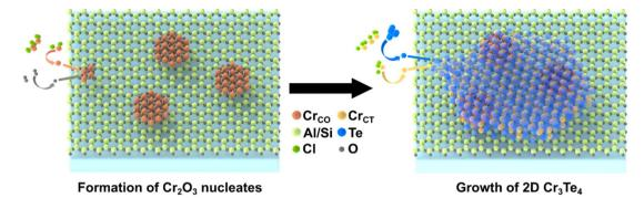
Fig. 4 A schematic diagram illustrating the proposed crystal growth model for epitaxially grown 2D  $Cr_3Te_4$  on the mica substrate. The process has two steps, with the first step being the formation of  $Cr_2O_3$  seed particles, and the second step being the growth of  $Cr_3Te_4$  based on  $Cr_2O_3/Cr_3Te_4$  interfaces.
