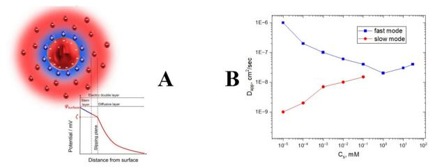
The general structure of a double layer (A). Relaxation time splitting for polyelectrolyte solution as a function of salt concentration (B)
