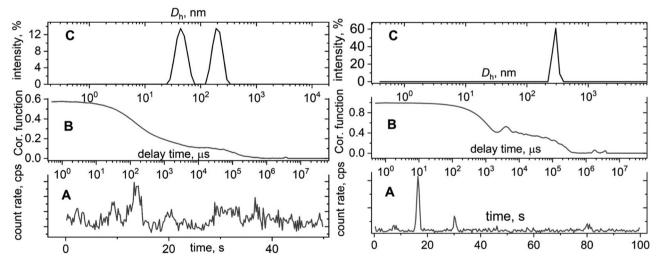
Fig. 2 Example of poor-quality measurements: typical count rate (A), correlation function (B), and D<sub>h</sub> distribution function (C) for samples containing dust or large aggregates (left); and for even the worst case of system sedimentation (right).
