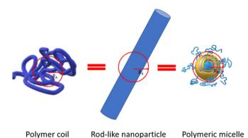
Fig. 5 Red circle represents hydrodynamic size as seen by DLS. Three different nano-objects with highly distinctive morphologies such as a polymer coil, rod-like nanoparticle, and a polymeric micelle have the same hydrodynamic size. This cartoon represents the fact that DLS is a "blind" method that provides the value of a diffusion coefficient converted later to hydrodynamic size. The mismatch depends on architecture and draining of the nanoparticles.
