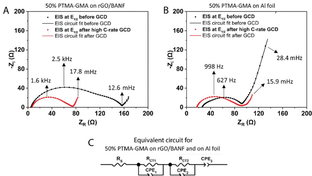
Fig. 5 EIS at the half-wave potential ( $E_{1/2} = 3.66$  V) for 50 wt% PTMA-GMA on (A) rGO/BANF and (B) Al foil before and after rate capability testing. (C) Fitted equivalent circuit for 50 wt% PTMA-GMA on rGO/BANF and Al foil.
