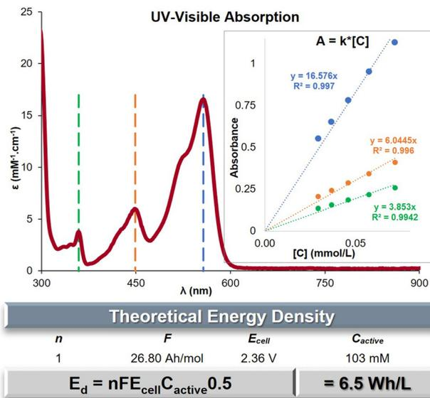
**Fig. 2** UV-visible absorption spectrum of  $\text{C}^+$  in CH<sub>3</sub>CN. Insert: Linear relation measure between concentration and absorption for a range of standards solution. Table: theoretical energy density numerical application.
