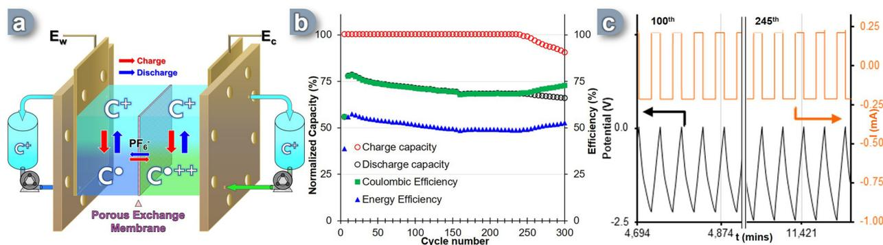
Fig. 3 (a) Scheme of the SORFB cell during cycling. (b) Plot of charge, discharge capacity (normalized to theoretical capacity), coulombic and energy voltaic efficiency vs. cycle number for RFB-cell cycling with tanks loaded each with 4 mL of 1 mM  $\text{C}^+$ , flow  $8 \text{ mL min}^{-1}$  per channel a 2C-rate for 300 cycles ( $\sim 9.5$  days). Each data point represents 5 cycles. (c) Monitoring of cell potential and  $I$  vs. times for cycle 100th to 105th and 245th to 250th.
