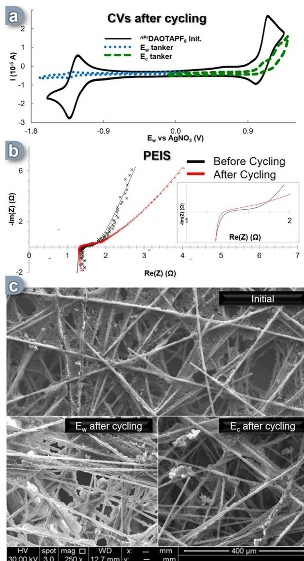
Fig. 4 (a) CVs of tank's solutions after 300 cycles ( $\sim 9.5$  days) and comparison with initial  $C^+$  CV. (b) PEIS of the cell in flow before and after 300 cycles (both at 0% SOC) from 1 GHz to 0.1 Hz with an amplitude of 10 mV. Insert: zoom on the fit intersection with the x-axis (c) SEM pictures of the carbon felt electrodes before and after cycling for both sides of the cell at magnification  $\times 250$ .
