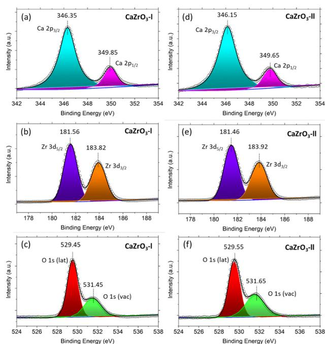
Fig. 5 XPS spectra of CaZrO<sub>3</sub>-I and CaZrO<sub>3</sub>-II: (a) Ca 2p-I, (b) Zr 3d-I, (c) O 1s-I, (d) Ca 2p-II, (e) Zr 3d-II, (f) O 1s-II.
