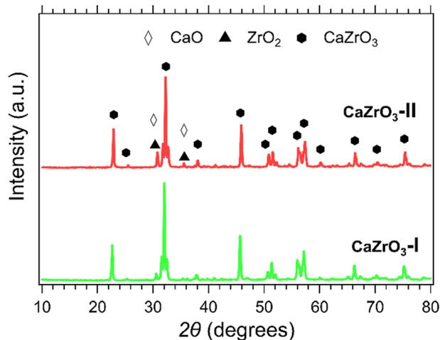
Fig. 3 XRD patterns of CaZrO<sub>3</sub>-I (green) and CaZrO<sub>3</sub>-II (red). Peaks of CaO are represented with the white diamond marker and ZrO<sub>2</sub> with the black triangle marker.
