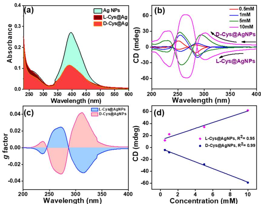
Fig. 4 (a) Comparison of the UV-vis spectra of Ag NPs, L-Cys@Ag, and D-Cys@Ag, (b) comparison of the CD spectra at various concentrations of L/D-Cys, (c) *g*-factor plot at 5 mM concentration of L/D-Cys, and (d) plot of ellipticity (mdeg) vs. concentration of chiral ligands (L, D-Cys) added to Ag NPs.
