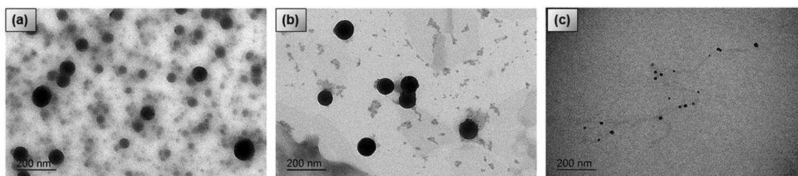
Fig. 3 TEM images of conjugated polymer/PC<sub>71</sub>BM heterojunction nanoparticles for the samples (a) P3HT-100, (b) PSiF-100, (c) PPV-100.
