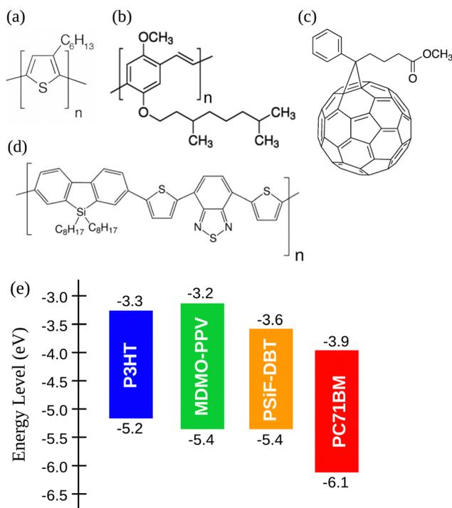
Fig. 1 Chemical structures of (a) P3HT, (b) MDMO-PPV, (c) PC<sub>71</sub>BM and (d) PSiF-DBT. (e) Energy level diagram of the considered polymers and fullerene.<sup>60–63</sup>
