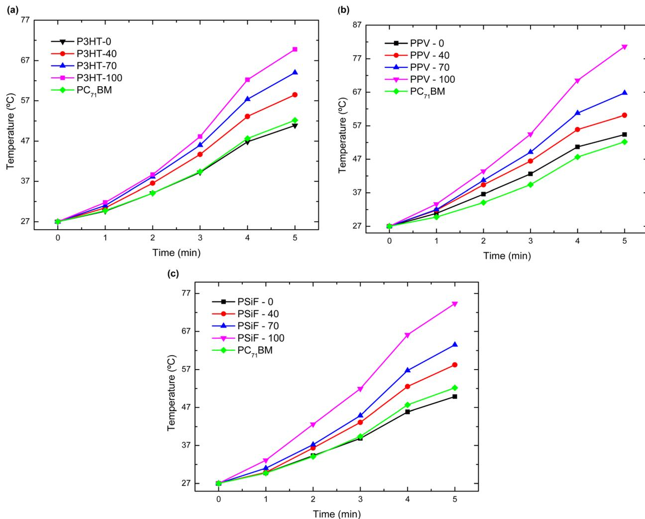
**Fig. 6** Final temperature in °C at the corresponding period of time samples were irradiated in isotherm, of pure conjugated polymer nanoparticles, pure fullerene PC<sub>71</sub>BM nanoparticles and polymer: PC<sub>71</sub>BM heterojunctions nanoparticles with fullerene doping amount of 40%, 70% and 100% for (a) P3HT, (b) MDMO-PPV and (c) PSiF-DBT.
