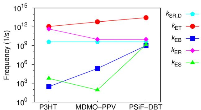
Fig. 8 Averaged rates over  $10^4$  runs of simulation for electron transfer, back, recombination and separation. A typical value of the singlet exciton recombination lifetime,  $\tau = 250$  ps, was used to obtain  $k_{SR,D} = 1/\tau$  for the polymers.
