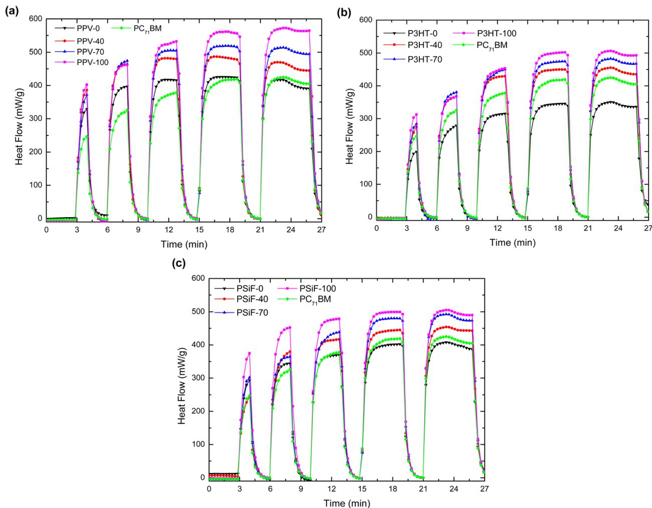
Fig. 5 DSC thermograms of samples under 532 nm laser irradiation in an isotherm of 27 °C, of pure conjugated polymer nanoparticles, pure fullerene PC<sub>71</sub>BM nanoparticles and polymer: PC<sub>71</sub>BM heterojunctions nanoparticles with fullerene doping amount of 40%, 70% and 100% for (a) P3HT, (b) MDMO-PPV and (c) PSiF-DBT.
