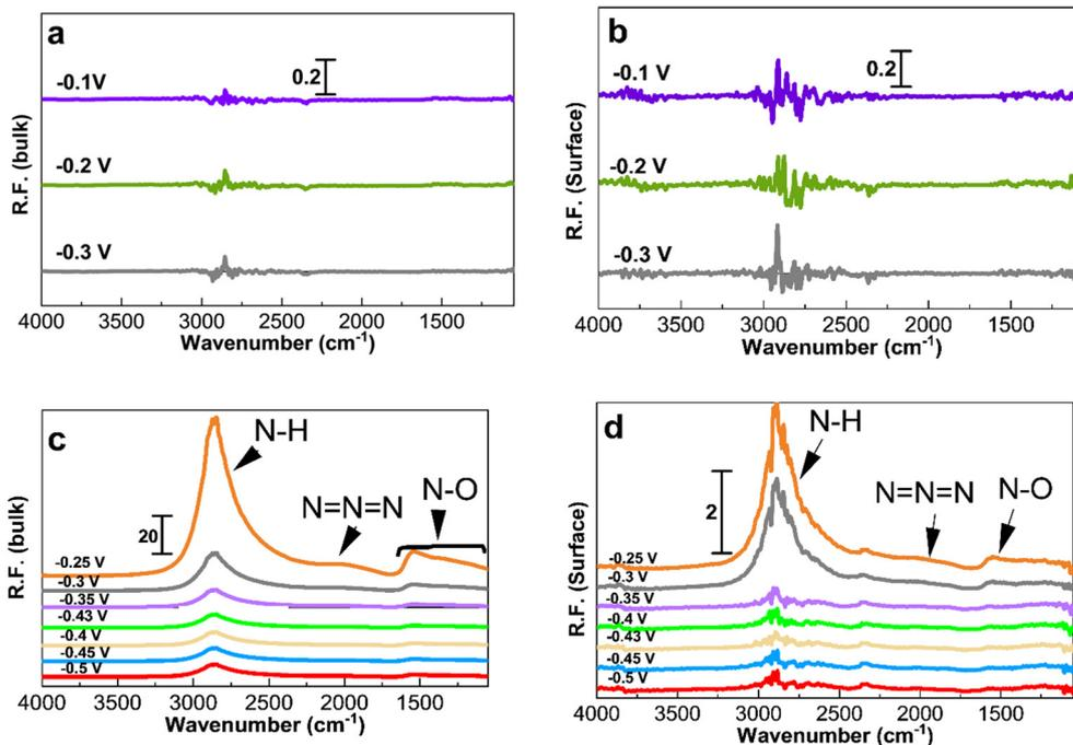
**Fig. 5** PM-IRRAS spectra (considering KOH at  $-0.4$  V as reference for processing the spectra) on Pt/C of 1.3 nm. (a and b) Spectra in 1 M KOH and (c and d) spectra in 1 M KOH + 0.5 M  $\text{NH}_4\text{OH}$ . The applied potentials in (c) and (d), as indicated in the figure, are  $-0.5$ ,  $-0.45$ ,  $-0.43$ ,  $-0.4$ ,  $-0.35$ ,  $-0.3$ , and  $-0.25$  V. The left hand side corresponds to the bulk of the electrolyte and the right hand side corresponds to the Pt surface.
