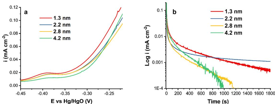
Fig. 3 (a) A comparison of the forward CV scans of Pt/C catalysts at  $v = 20 \text{ mV s}^{-1}$  and (b) chronoamperograms of Pt/C catalysts at  $-0.3 \text{ V}$  in  $1 \text{ M KOH} + 0.5 \text{ M NH}_4\text{OH}$ .
