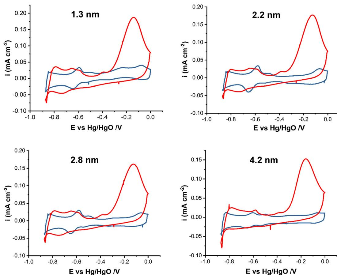
**Fig. 2** Cyclic voltammograms of Pt/C catalysts of various average sizes as indicated in the figure in 1 M KOH (blue line) and in 1 M KOH + 0.5 M NH<sub>4</sub>OH (red line) at 20 mV s<sup>-1</sup>.
